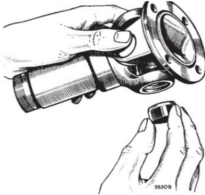
Fig. G.3 Showing the manner of withdrawing the needle bearing after it has been partly withdrawn. When bearings are removed or replaced they should be held vertically to prevent the needle bearings from being displaced
