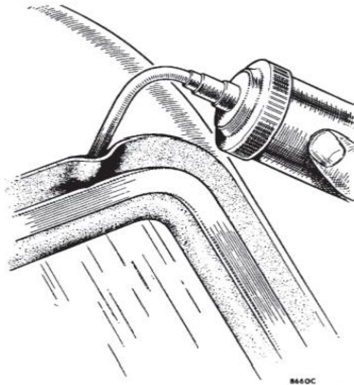
Fig. S.5 Showing the use of a pressure gun to apply Seelastik
