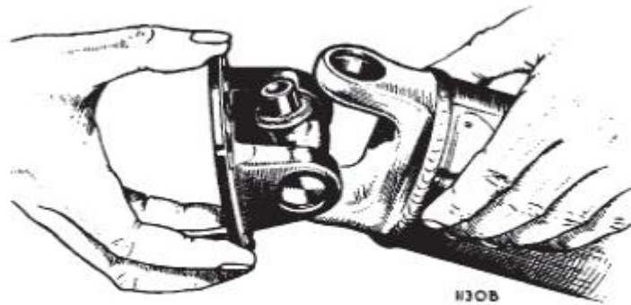
Fig. G.4 When the needle roller bearings have been withdrawn from opposite sides of the spider, the joint can be separated as shown
