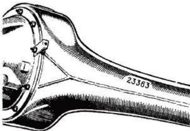
Rear Axle Number. Stamped on the front of the left-hand rear axle tube
