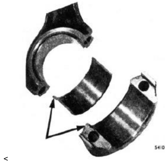
Fig. A.12 A connecting rod bearing. Note the bearing locating tab
