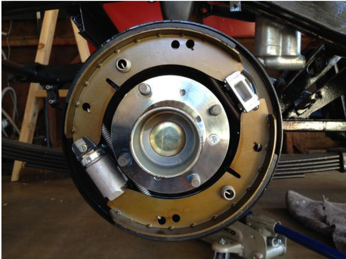
Fig. M.5 A rear brake assembly. (wire wheel)
