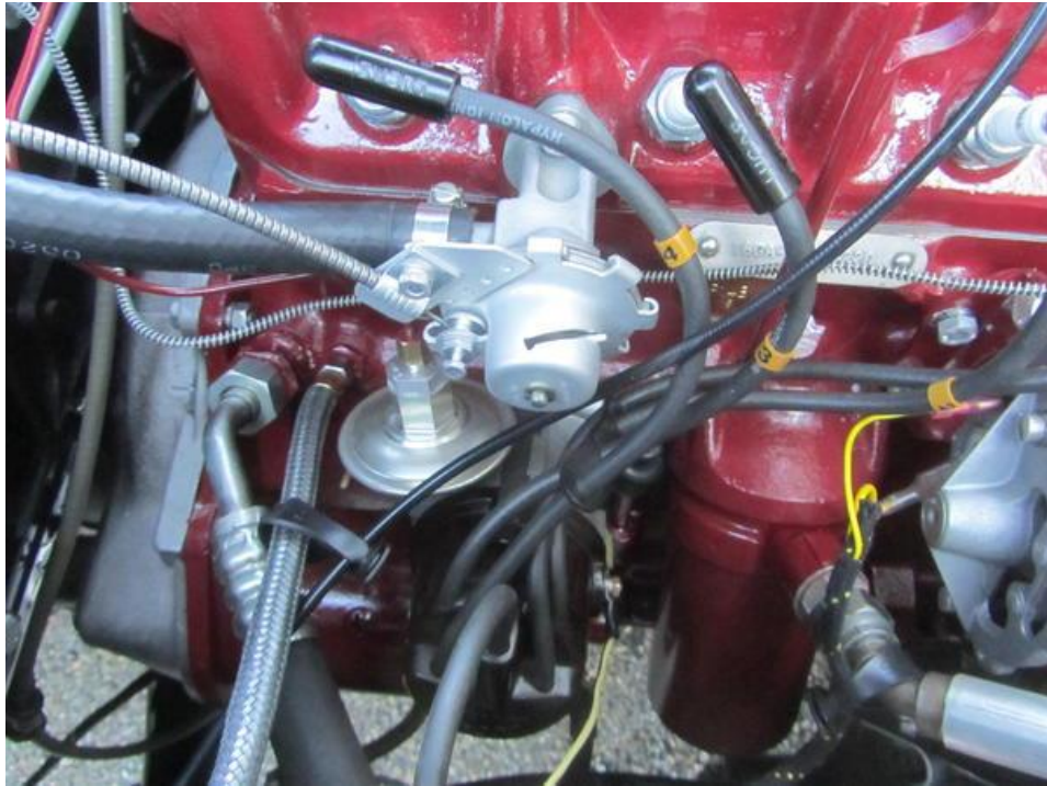
Fig. S.4. The position of the water valve lever with the control pulled out to the "Min." position.
