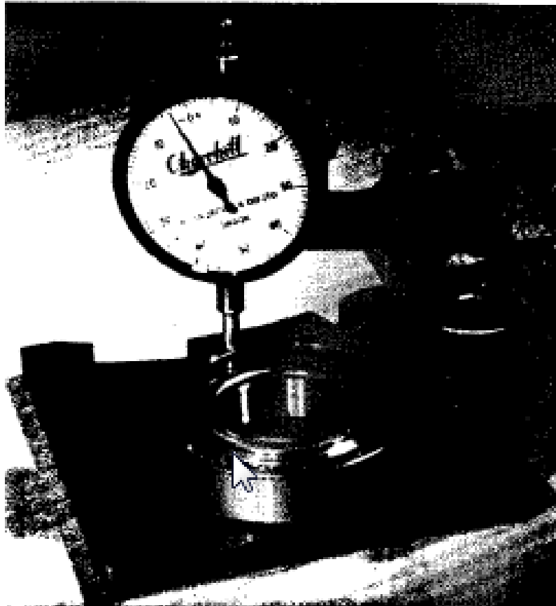
Fig. H.7 With the gauge set to zero, place the bearing on the surface plate with the outer ring thrust face down, and take a reading while the indicator foot contacts the inner ring
