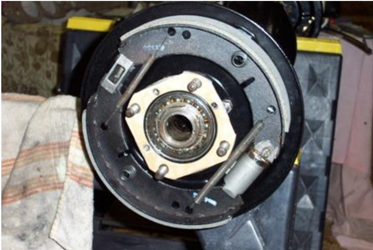
Fig. M.5 A rear brake assembly. (disc wheel)
