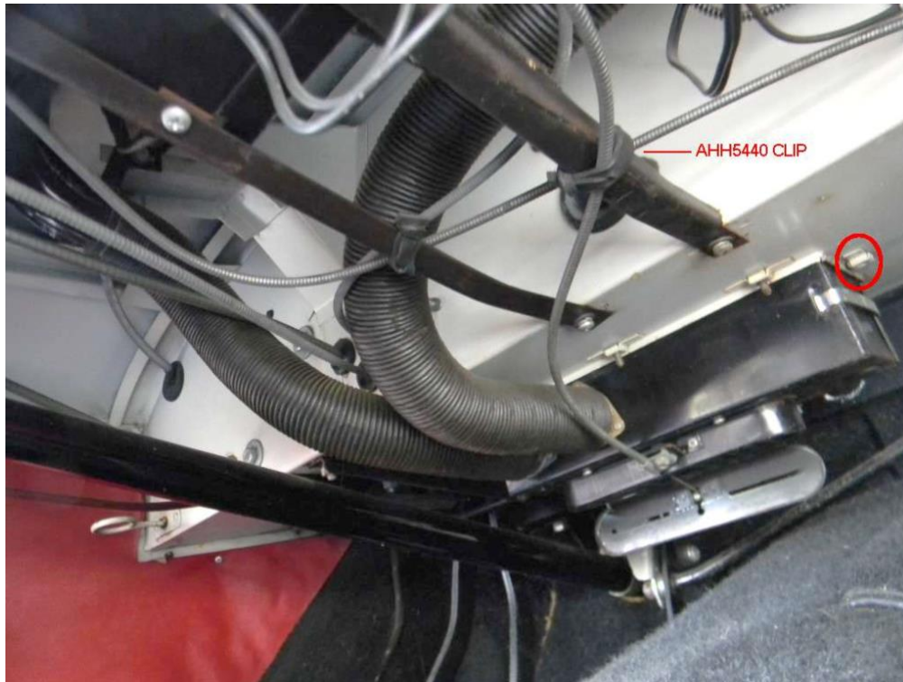
Fig. S.6. Showing the general layout of the heater controls and demister tubes inside the car.
