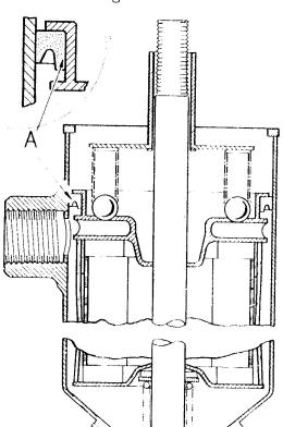
The seal used (Part No. 17H847) is moulded, as shown on left, and this replaces the 'O'-sectioned packing ring without change in part number.
