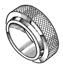
To ensure the correct positioning of the gearbox front cover (which carries an oil seal) it is important that the cover is fitted concentric to the first motion shaft if oil leaks are to be avoided. To help in this direction, this Service Tool 18G598 has been designed, and is considered to be essential when the front cover has been removed for any reason.
