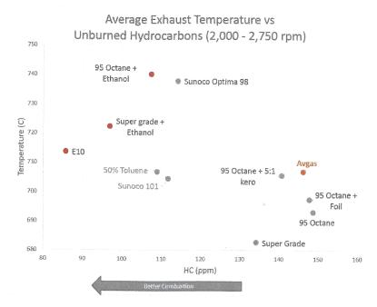
reduction is not caused by the kerosene failing to burn properly; the level of unburned hydrocarbons in the exhaust (141 ppm) was slightly less than that of petrol on its own (149 ppm), suggesting people's worries about the kerosene not burning are unfounded.
