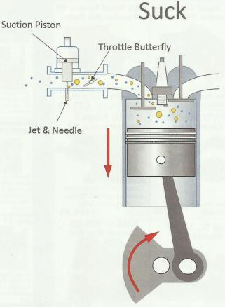
flows through the carburettor. Its height is a measure of the volume of air flowing into the engine and by withdrawing the tapered needle from the jet, it allows more fuel into the air stream. In this way the SU carburettor is able to accurately control the air/fuel ratio.
