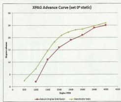
around 5° too retarded below 4000rpm, supporting general observations that it is necessary to advance engines when using modern fuel. Unfortunately, the shape of the original curve is wrong. Increasing the standard advance to 5° static improves the timing up to ~3000rpm, beyond which the engine is too advanced.
