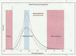
these two effects, indicating cyclic variability is a significant factor during the Bang cycle of the XPAG engine.
