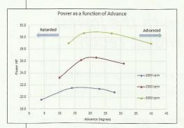
of power output to ignition timing. At 3000rpm, advancing or retarding the ignition by as much as 10-15 degrees only changed the power output by ~5%. This suggests the combustion profile is very spread, as is discussed below.
