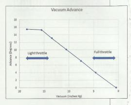
centrifugal advance is needed. On later cars this is achieved using the vacuum pod on the distributor which is connected to the inlet manifold. A light throttle setting reduces the pressure in the inlet manifold causing the pod to advance the ignition timing. Earlier cars do not have a vacuum advance.
