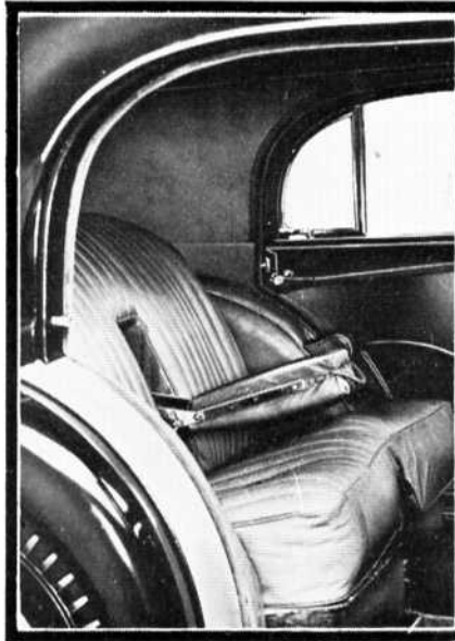
Side and centre arm-rests are provided. Note the no-draught ventilation panels.
