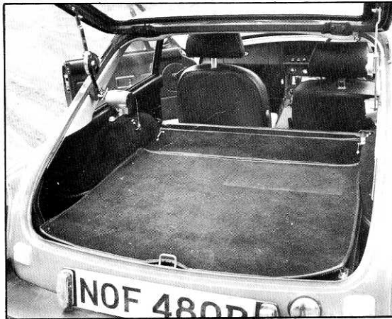
The modest boot extends usefully in size when the rear seat back is folded and loading is easy through the deep tailgate. Below: Spare wheel and jack stow under the floor
