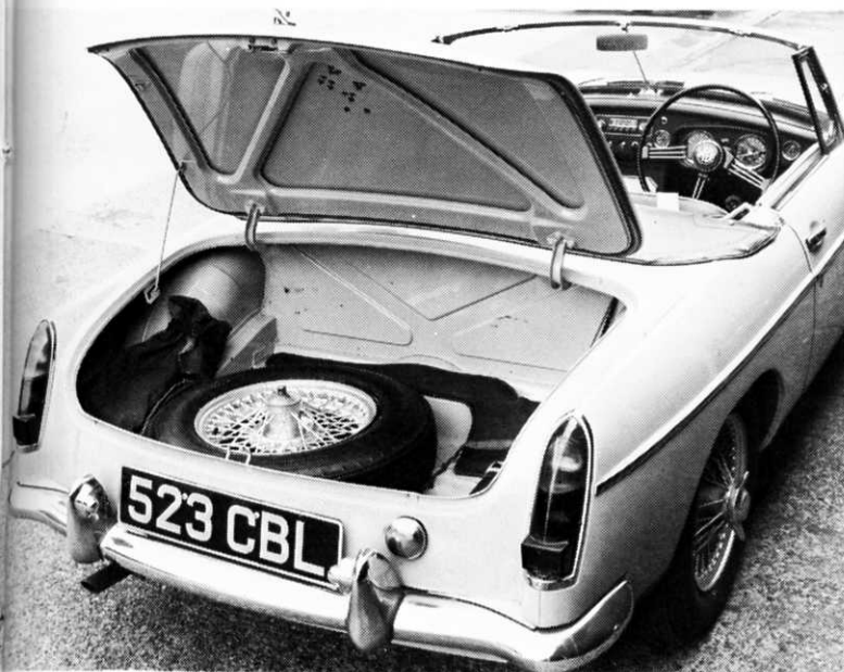
An inconvenient prop has to be fixed in position to hold the boot lid open. Luggage space is severely restricted by the positioning of the spare wheel
