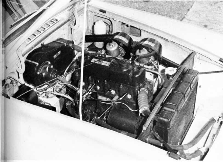
Apart from the distributor, which is obscured by the pipes to the oil cooler, all components are commendably accessible. The oil cooler, which is optional on home market cars, is visible ahead of the radiator
