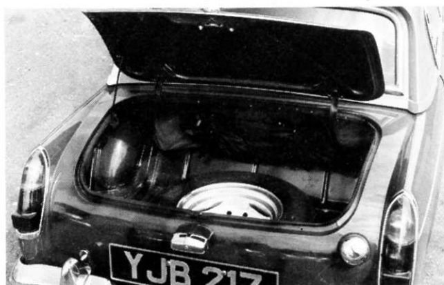
The toolkit comprises a side-lifting jack, a wheelbrace, and a socket spanner for the sparking plugs. Storage bags are provided for the hood
