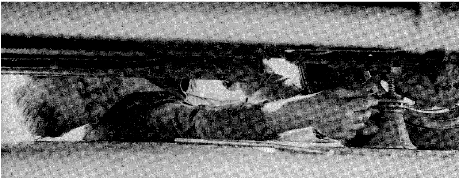
Putting the MGA jack into position
