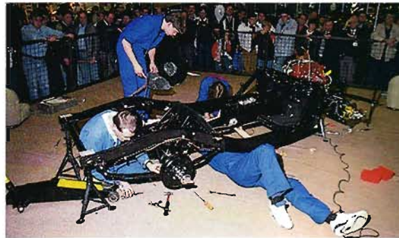
Above, far left and left, restoration in progress – 1961 MGA 1600 rebuilt from scratch in two days by Heritage organisation in time to be driven by Tony Dron on 1992 Monte Carlo Challenge
