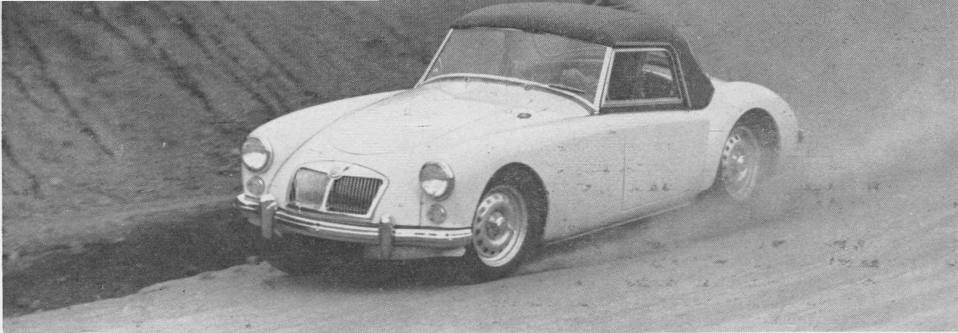
Slicing through a dirt-covered downhill, the car depends on its big, meaty anti-sway bar and RS-5 tires for stability.
