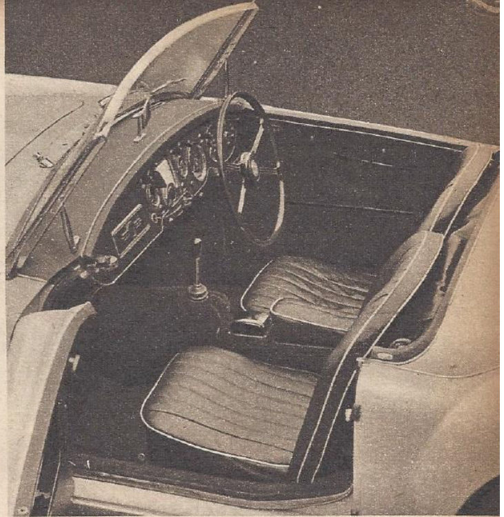
Both the facia and the decking below the screen are now covered in a grained black plastic material which effectively prevents reflections at night. A praiseworthy addition is a headlamp flasher on the extreme right of the facia. Upholstery is in leather and the floor is carpeted
