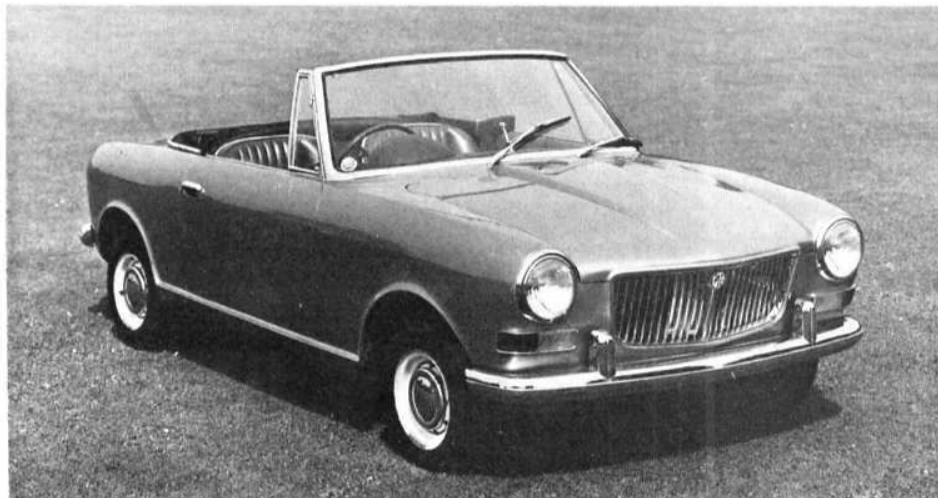
Below, a variation on the ADO34 scheme, done by Abingdon stylists. Note similarities to MGB (and the MGB bonnet left of the picture). Left, below, there was room enough for two back seat passengers in the ADO34, but a metal tonneau would also have been supplied.
