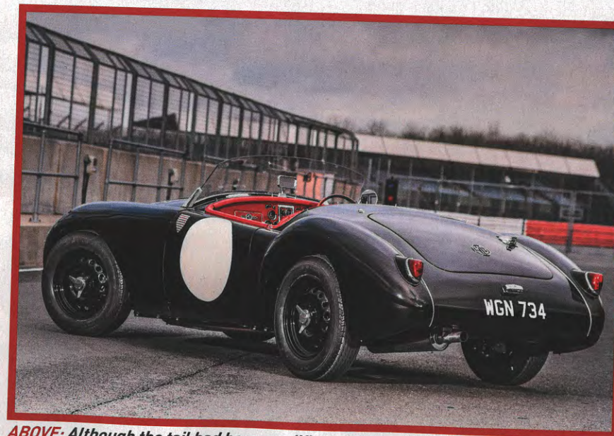
ABOVE: Although the tail had been modified by later owners, the original curves were rebuilt in aluminium because that is how it had been raced from new.
