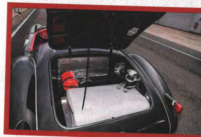
ABOVE: The large fuel tank in the boot had originally been adapted from that found in a Commer van.
