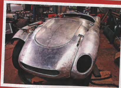
The streamlined front end that Paul Fletcher had commissioned back in 1958 was destroyed by fire and had to be painstakingly recreated by hand from aluminium.
