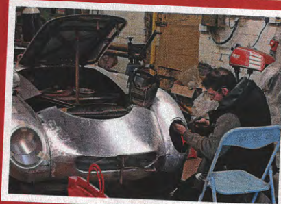
The streamlined front end that Paul Fletcher had commissioned back in 1958 was destroyed by fire and had to be painstakingly recreated by hand from aluminium.
